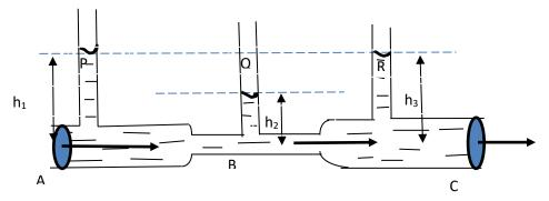
Since liquid pressure is given by the equation  $h\rho g$ , then the liquid columns at A and C are such that  $h_1=h_3$ . Therefore, the liquid pressure is equal at A and C. But  $h_1>h_2$ , where  $h_2$  is the height of the liquid column at B. This means that the liquid pressure at A and C is greater than that at B.
