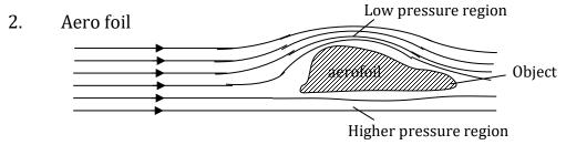
The wing of an aircraft has a curved upper surface and a flat under surface. This compels the air passing over the top of the wing to travel a longer distance resulting in a higher air velocity than that below the bottom surface.
