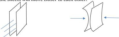
When a stream of fast moving air is blown below a thin sheet of paper held horizontally on pieces of wooden blocks, the paper will move downwards. If the air is blown above the same paper, it will move upwards.
