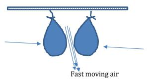
When a stream of fast moving air is blown between two thin sheets of paper held vertically close to each other, the sheets will move closer to each other.
