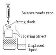
The displacement can is filled with water up to its spout and some time is allowed for the water to stop dripping.
