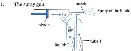
When the piston is pushed in, it forces the air in the cylinder to move with a high velocity over the tip of the tube, T. This causes the air inside the cylinder to fall below that in the liquid reservoir. The pressure acting on the liquid surface forces the liquid to rise up the
