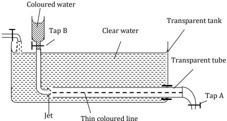
A transparent tank, fitted with a horizontal transparent tube is filled with water from a tap. Tap A controls the rate of flow through the horizontal tube while tap B opens for the coloured liquid.
