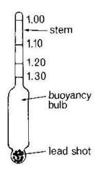
It consists of a longer glass tube with a bulb at the bottom filled with mercury or lead so that the hydrometer floats up right. The stem is long and thin and is graduated. The thin stem means that the hydrometer is sensitive.
