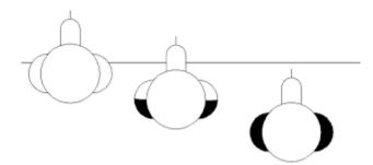
When air is pumped into the tanks, the average density of the submarine falls until it's the same or slightly less than that of water around it. The submarine therefore stays at one depth or rises to the surface.
